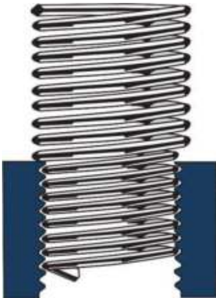
Recoil insert in semi-installed position
